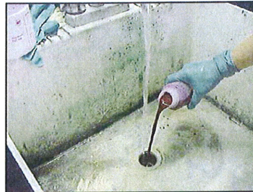
Figure 63: Dye Testing Plumbing (NEIWPCG, 2003)
