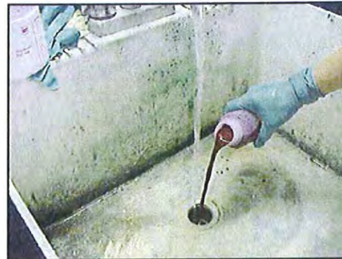
Figure 63: Dye Testing Plumbing (NEIWPCG, 2003)
